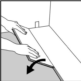
Place the second floorboard **TIGHT** to the short end of the first board in the second row and fold down in a single action movement.
