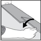
Place 5/16" spacers to provide for the expansion space along the wall.
